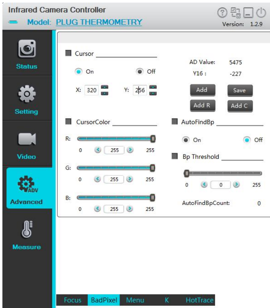
Fig. 4-34 Defective pixel correction interface
